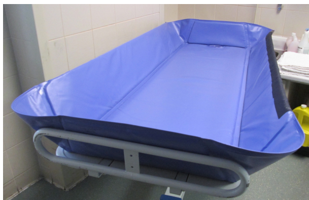
Figure 2. Preventative application of CleanPatch to high wear area (9 months after application)
